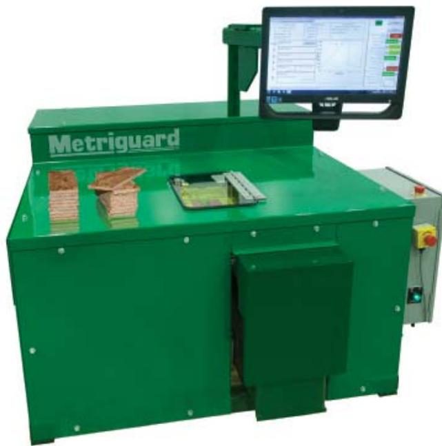
Rail Shear Tester with computer controls, safety door and emergency stop
